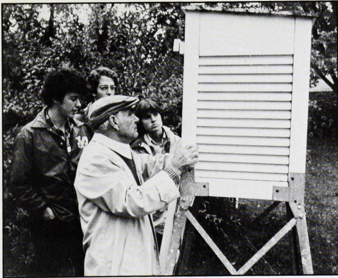
While the equipment has become somewhat more sophisticated over the years, the routine has varied little. Every morning the precipitation is measured and the highs and lows recorded. Photographs by Erik Borg.
